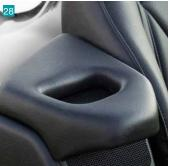
**Pillion Armrest Extension Set** Increase your pillion's comfort with these armrest extensions designed to allow the sound of the rear speakers (when fitted) to pass through uninhibited.
