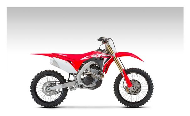
Model updates: The new CRF250R links up its strong bottom-end torque and potent topend power with a much bigger hit of both through the mid-range; the 19YM CRF450R frame and swingarm now provide the basis for the chassis, with revised damping for the Showa suspension.
