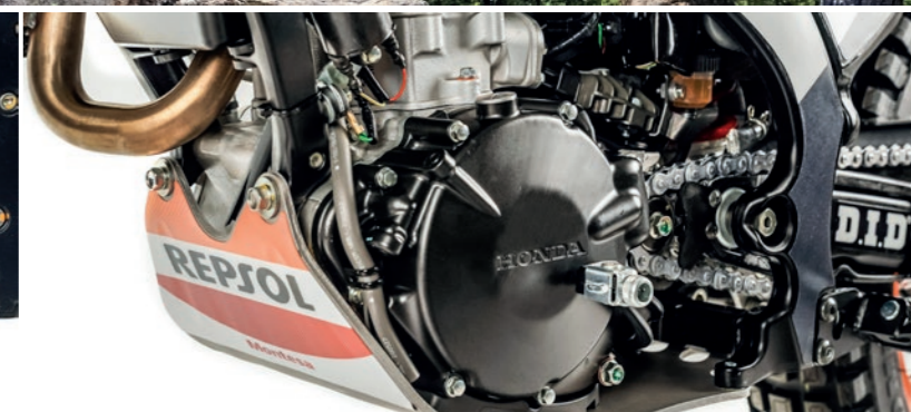
Fuel-injected, four-valve 298cc four-stroke engine
