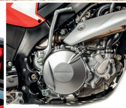
Fuel-injected four-stroke four-valve 259cc engine
